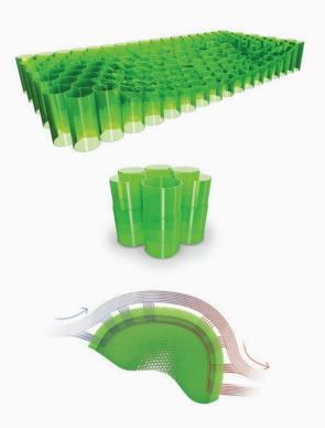
Developed as an energy absorber in the aerospace industry, cylindrical structures were found to be one of nature's strongest forms; a form that could offer the greatest impact absorbtion for a given length. Koroyd® utilizes cylinders to create a structure that Traditional materials act like a spring which stores energy and then releases it, Koroyd® is a true energy absorber which converts the kinetic energy by crumpling. This translates into better absorption of impact energy.
